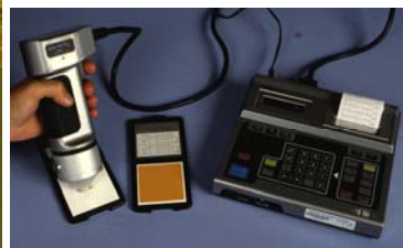
Example of a reflectance colorimeter Values define a point in a 3-D color space
