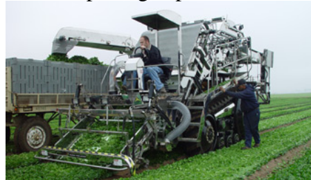
Mechanical harvest of young spinach for washed and packaged product
