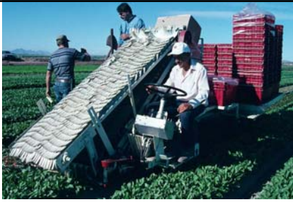
Mechanical harvest of young spinach for washed and packaged product
