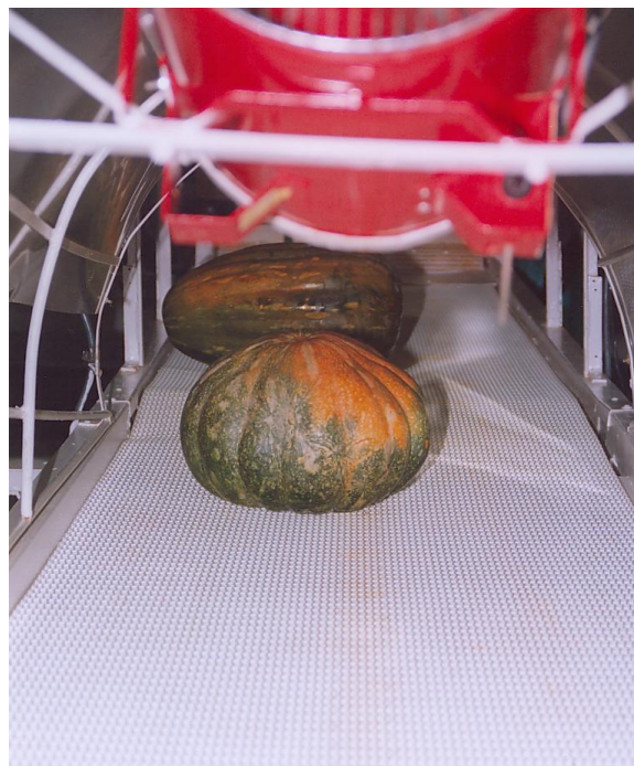
Figure 31: Forced air drying of sanitized fruits
