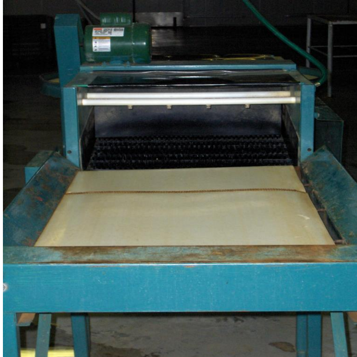
Figure 16: Fruits are wiped with clean water and placed on sanitized padded conveyor belt
